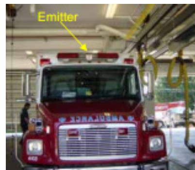
(c) Emitter source on fire truck
