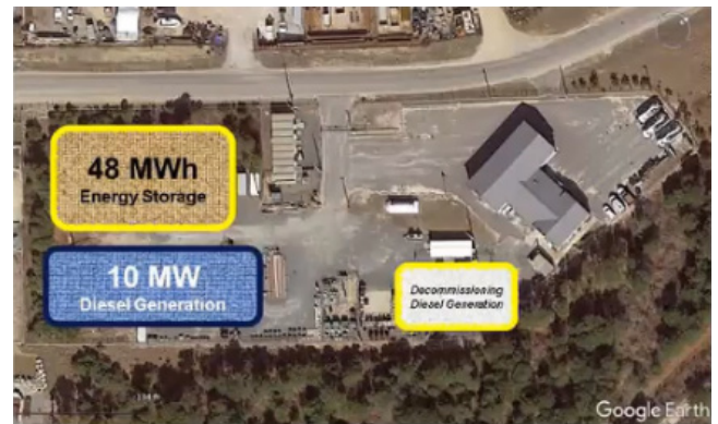
Fig. 7: Nantucket Island's project, hybrid option: Combustionengine together with a storage
